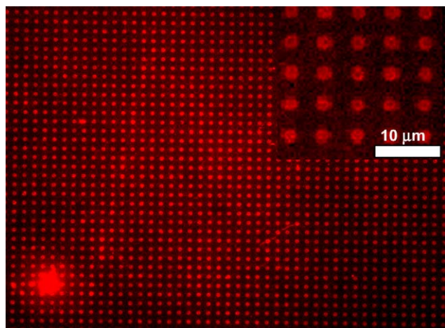
Figure 4. Fluorescent picture of a micropatterned gold surface with BAT showing the interaction between streptavidin labeled with a fluorescent dye and biotin.
